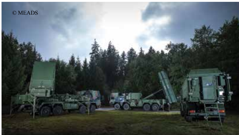
German configurations, a MEADS Multifunction Fire Control Radar, launcher, and battle manager appear together near Freinhausen, Germany.
