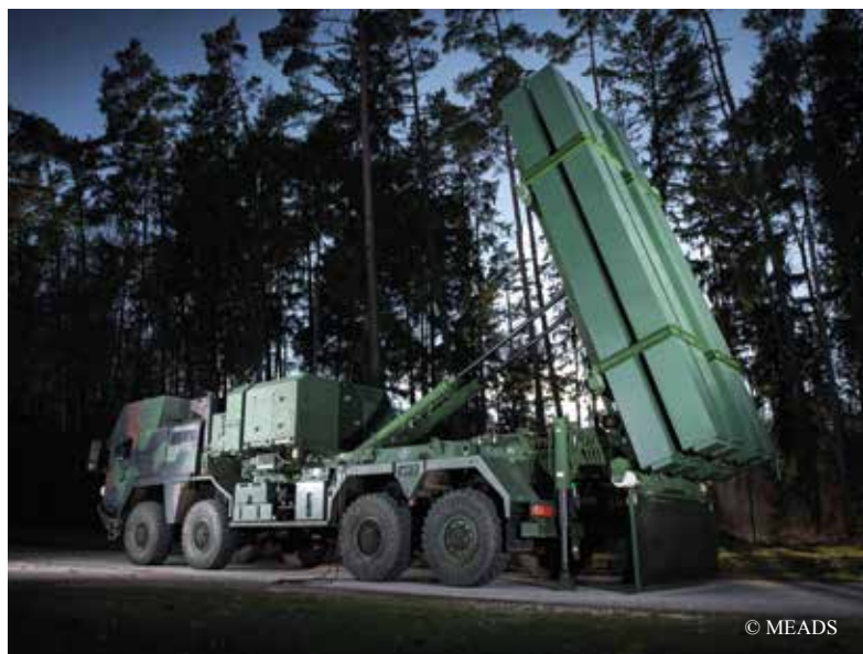
A MEADS launcher in the German configuration is A400M transportable and can engage and defeat targets attacking from any direction
